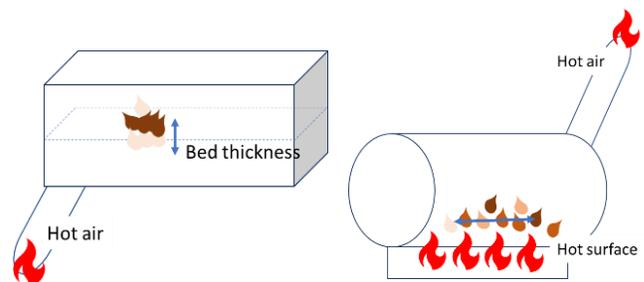
Figure 1. Roasters (fluidized bed roaster left, drum roaster right).
