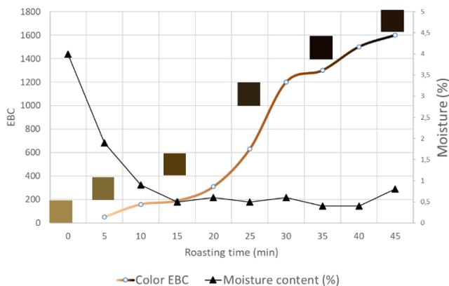
Figure 6. Impact of roasting at 240°C on color and moisture content of kilned malt.
