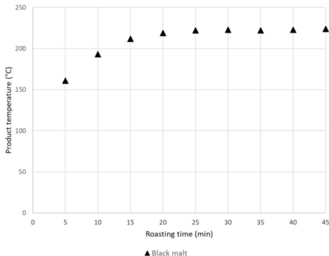
Figure 7. Impact of roasting at 240°C on malt temperature.
