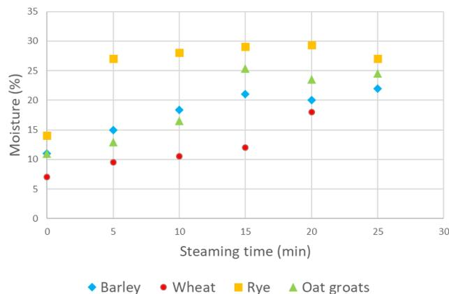
**Figure 10.** Impact of steaming at 100°C and 10% steam on different grains moisture.
